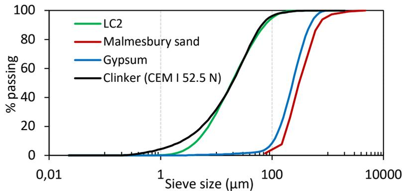
Fig. 1. Particle size distribution of LC<sup>2</sup>, Malmesbury sand, Gypsum, and CEM I 52.5 N
