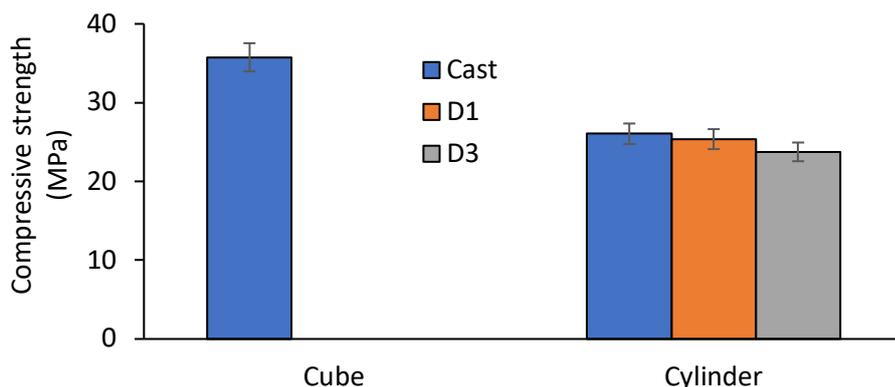
**Fig. 3.** Compressive strength development of LC<sup>3</sup> FR-3DPC specimens after 28 days curing
