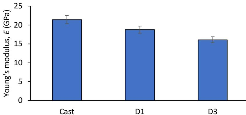
**Fig. 5.** Young's modulus results for LC<sup>3</sup> FR-3DPC specimens at 28 days of curing
